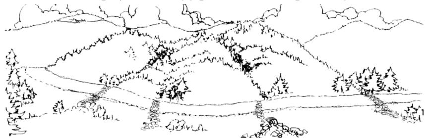
Provide frequent ditch relief with x-drains or rolling dips. Place outlets in natural drainages if possible. Road building or other construction near a stream, river or estuary can create serious fish habitat damage if the work is not done properly.
